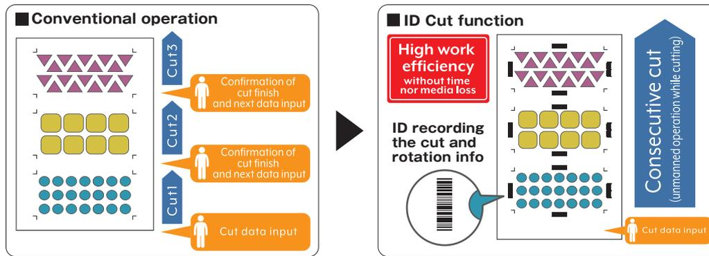
Print data as well as register mark with ID can be printed out by JV300-130/160 Plus simultaneously.
